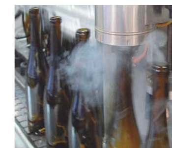
Bottle inerting with liquid nitrogen
